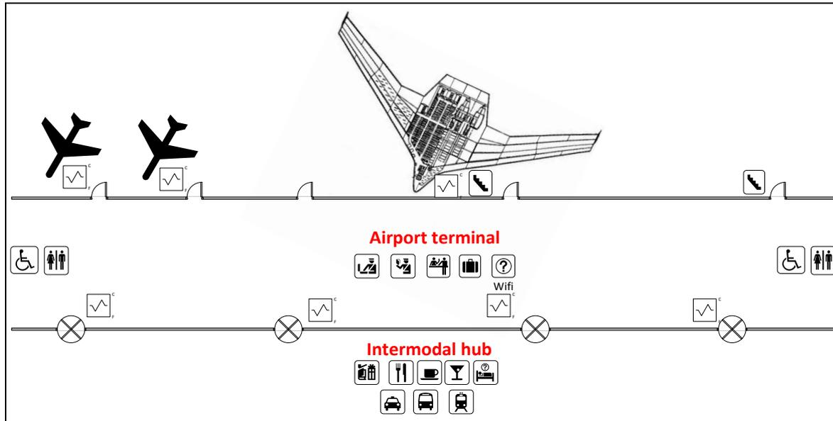
Figure 16: The possible new layout of a lean terminal
