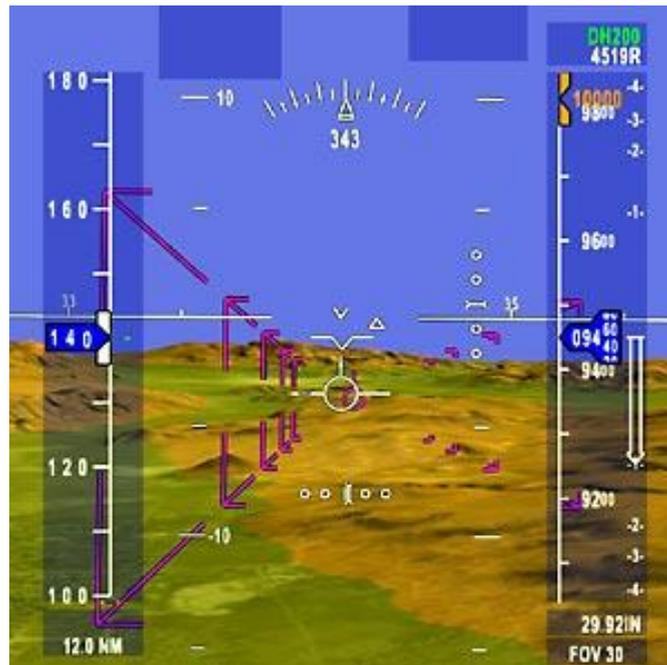
Figure 14: Example of a Synthetic Vision display
