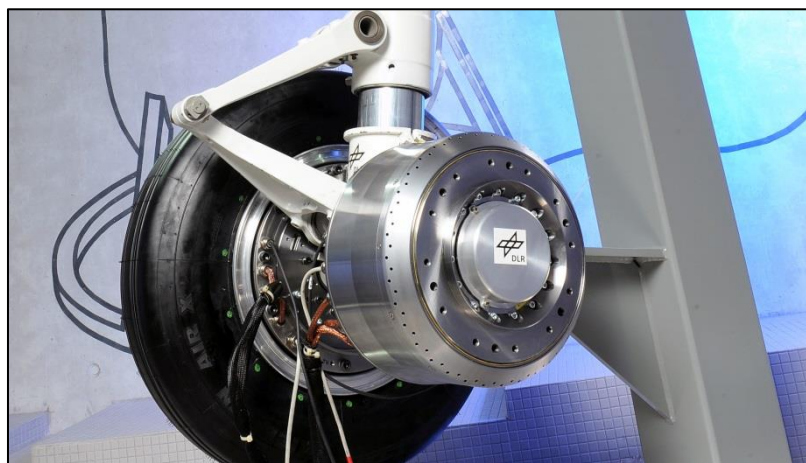
Figure 18: Nose gear with electrical engine, source: [62], © DLR.
